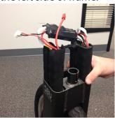
23. Reconnect Battery Positive Connector (Red). Replace electrical tape around connector.
