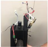
35. Reconnect Battery Positive Connector (Red) Replace electrical tape around connector.
