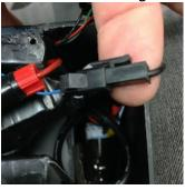
29. Pull out the motor cable so you can move the battery freely.
