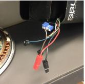
11. VERY CAREFULLY remove one of the BMS Ribbon Cables (White Connector). Use the side without the hot glue
