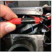
36. Reconnect Battery Half Connector (Green). Replace electrical tape around connector.
