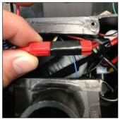
7. Disconnect Top Plate Power Switch Connector (Black).
